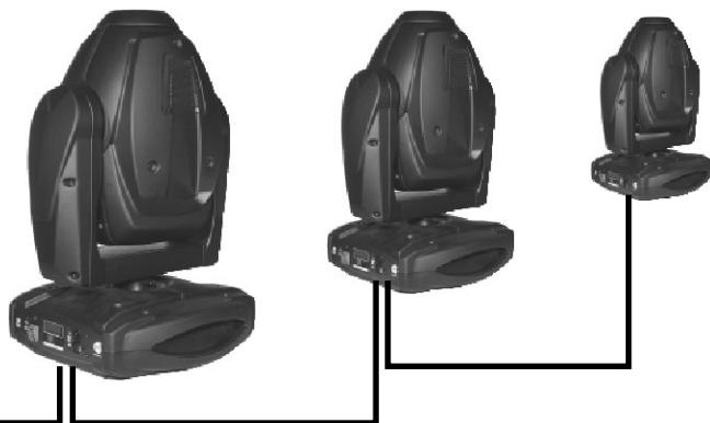
For installations where long distance DMX cable connections are needed, we suggest to use a DMX terminator.
