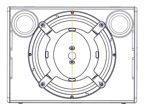
**3.** Secure the waveguide to the cabinet with the provided 100546s
