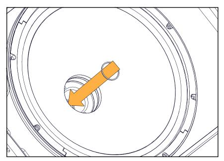
2. Position the waveguide.
