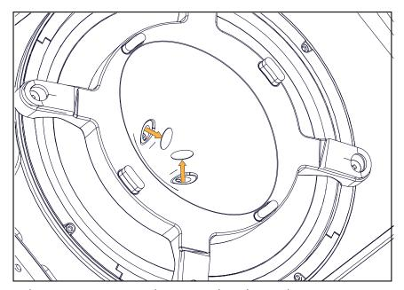
**2.** Remove the two screws securing the waveguide to the speaker.
