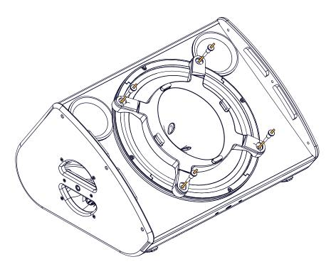
**4.** Secure the waveguide to the speaker with the provided 100547s
