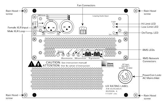
User Panel with RMS option and Polarity and Attenuaing Audio Input Module
