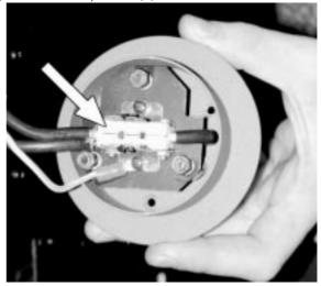
4) Insert the lamp in the lampbase. The lamp is manufactured from quartz glass and should be handled with care; always adhere to the instructions supplied in the lamps packaging. Never touch the glass directly, use the tissue provided in the lamps packaging. The GY 9,5 lampholder is asymmetrical in construction, with one lamp pin larger than the other. DO NOT USE UNDUE FORCE. In case of difficulty, inspect for physical damage and then repeat the installation procedure.
