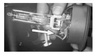
5) Replace the lamp assembly (B) into its original position and replace the screws (A) which were removed previously.
