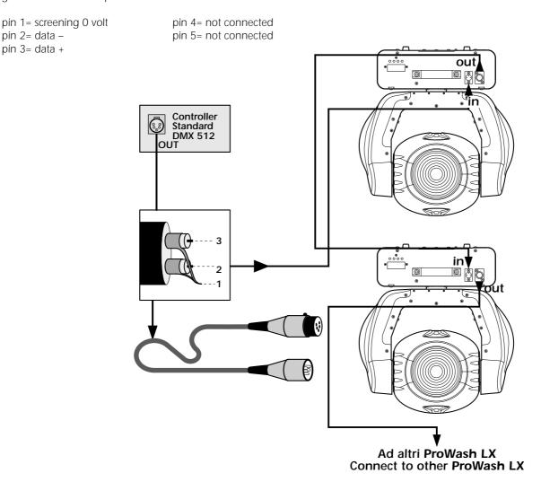
Ensure that all data conductors are isolated from one another and the metal housing of the connector.
