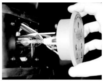
**Attention:** we recommend that replacement lamps be realigned in the optical path of the lamp so as to avoid any accidental overheating of the internal components of the fixture. This procedure is describe in the section of this manual entitled **"Aligning the lamp in the optical path"**.
