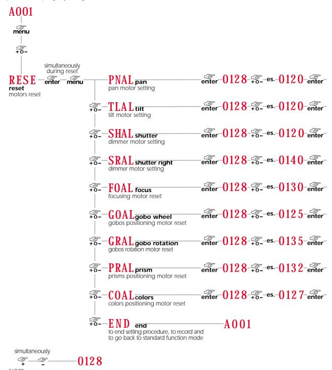
To speed up setting/alignment procedure, press simultaneously keys + and -; the display will automatically go to 128
