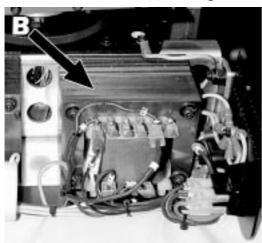
3) Select the operating voltage from the 100, 115, 208, 230 and 245V options by moving the cable n° 7 to the required voltage. To ensure correct positioning of the cable, refer to the label located on the transformer.
