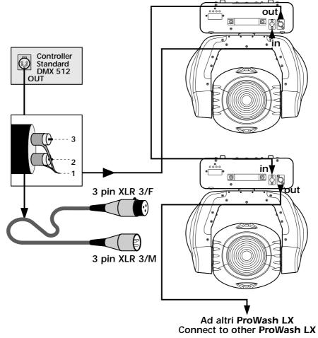
Should your DMX 512 controller utilise only XLR 5 sockets, the polarity of pins 1, 2 and 3 must be preserved as shown in the diagram. Do not connect pins 4 and 5.
