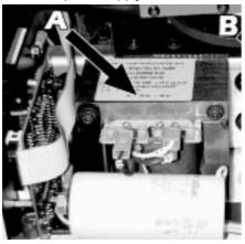
2) Select the required frequency from between 50 and 60Hz by moving cable n° 11 to the correct option. To ensure correct positioning of the cable, refer to the label located on the power supply.
