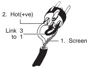
Balanced 3 pole Jack      Unbalanced 3 pole Jack
