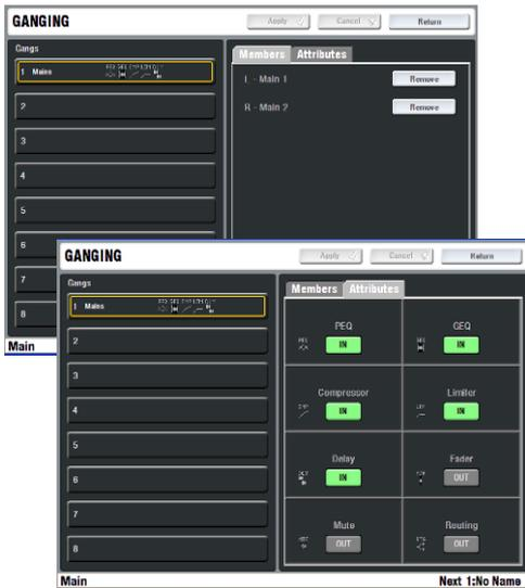
Ganged channels must be compatible input or mix types. Up to **8 gangs** can be assigned with **up to 8 channels each**. The parameters available to be ganged are known as the 'attributes'. These include processing such as EQ and dynamics, delay, routing levels and assignments and mutes.
