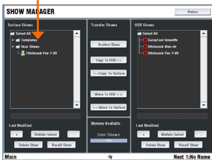
Shows are stored on the TouchScreen computer within the Surface or on the Editor laptop and can be transferred between systems using a USB key.
