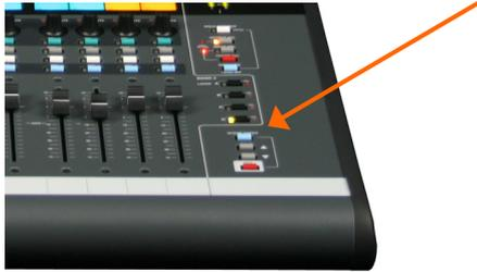
**Scene Recall Safes** lets you make selected input channels, mix and DCA masters 'safe' so that their parameters are not overwritten when a Scene is recalled. Hold down the Surface **SCENE SAFES** key and press the strip **MIX** keys on channels you want to make safe. The **SAFE** icon in the strip LCDs turns on for channels made safe. You can also right click the MIX or SEL button in the channel windows in **Editor** to access the Safe setting.
