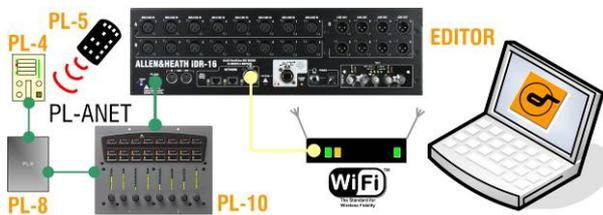
**Operating without a Surface** Leave your Surface at home and control iLive using just your laptop and iPad for compact or discreet mixing situations. You could add one or more PL Series controllers if you want to assign some physical control, for example important channels, DCAs or master levels.
