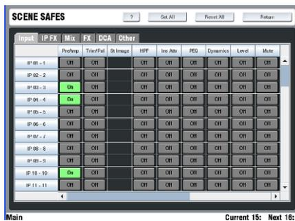
Navigate the tabs to find the parameters and channels you wish to make safe. Touch a channel number in the left column to make all parameters for that channel safe. Touch a parameter button in the top row to make that parameter safe across all channels. Use the buttons at the top to set or reset all items on that page.
