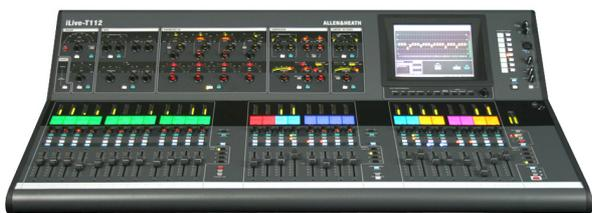
The **Surface** is simply a **network controller** for the MixRack. It has a built-in interface for local audio which is transported to and from the MixRack via the ACE connection along with the Ethernet control. Each bank of faders has 4 or 6 layers providing a total of 72, 80 or 112 control strips depending on Surface size. These strips are freely assignable as inputs, mix masters or DCAs in any combination.
