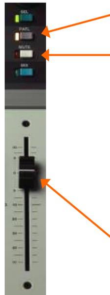
Pressing a **DCA master PAFL** key mixes all assigned channels to the PAFL monitor.
