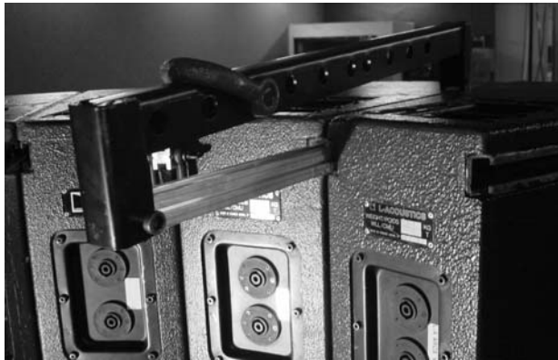
(7) BUMP3 slides into position from the rear
