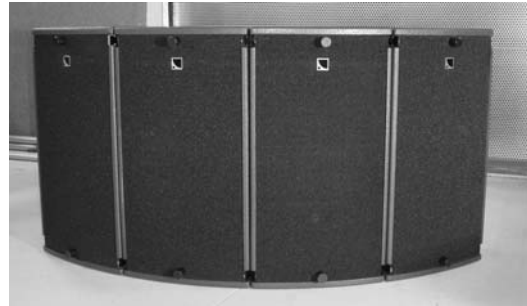
(4) Front dolleys removed (note: logos oriented upwards indicate that ARCS are inverted for -40 / +20 deg coverage)
