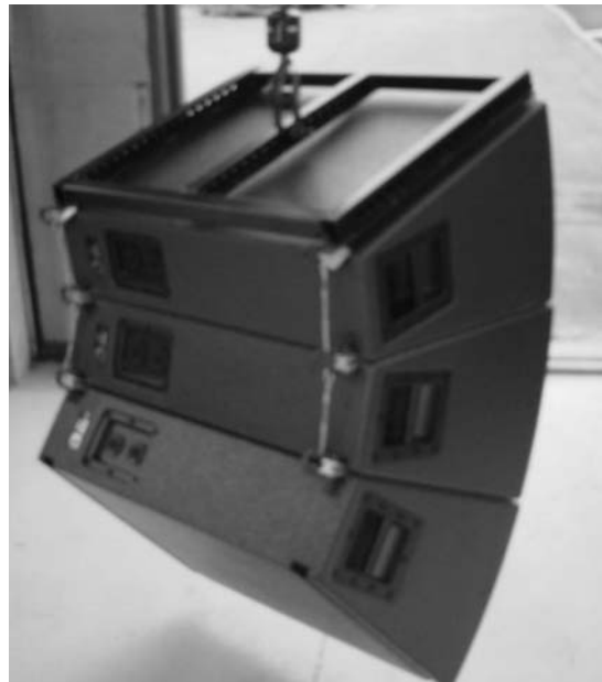
(14) The final flown assembly (rear view)
