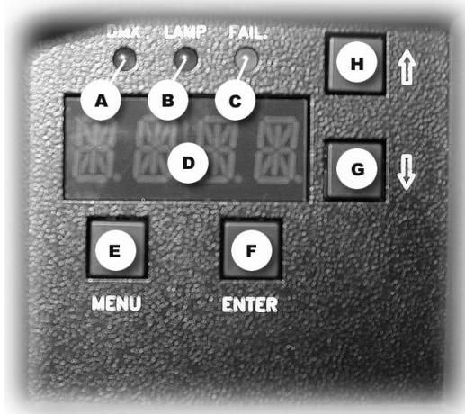
On the front panel of **MP700 Wash** you'll find a section for the additional functions and for setting the projector.
