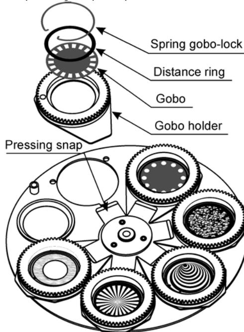
**CAUTION!** *The gobo holder with the magnet must be placed in the same gobo position as it was placed before gobo replacement!*
