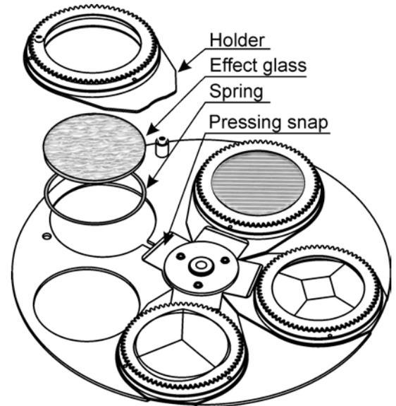
**CAUTION!** *The effect glass holder with the magnet must be placed in the same glass position as it was placed before glass replacement!*
