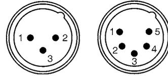
If you are using the standard DMX controllers, you can connect the DMX output of the controller directly with the DMX input of the first fixture in the DMX chain. If you wish to connect DMX controllers with other XLR outputs, you need to use adapter-cables.
