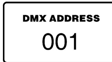
The main menu of the control panel is accessed by pressing [ENTER] button. To browse through the menu, rotate [RNS] wheel. To select a function or submenu, press [ENTER] button. Presetted options are displayed negative.
