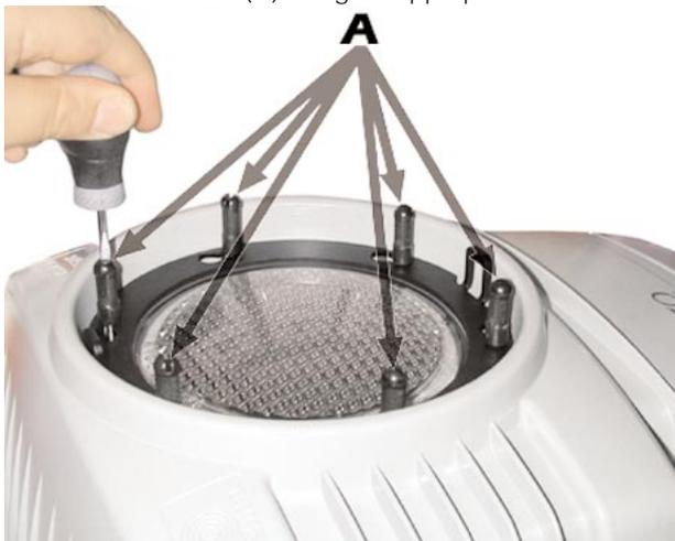
2) Rotate and remove the fixing ring.
