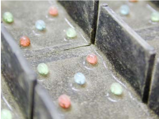
Image 6-1 LED's and shaders covered with dirt.
