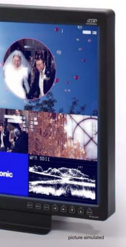
The AG-HMX100 is a compact, all-in-one, digital AV mixer with a built-in HD/SD multi-format\*1 video switcher, audio mixer, frame synchronizer and digital effector. It serves as an audio/video switcher, adds a variety of effects, and transmits signals - all by itself.
