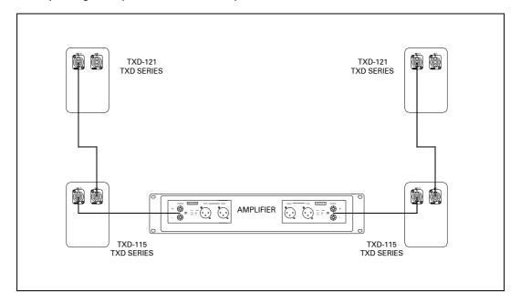
Connect the amplifier output to the Speakon INPUT socket on the bass enclosure.
