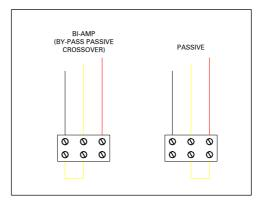
Mode selection is determined by the position of the wire links on the connector block. To bypass the internal passive crossover, connect the yellow link wire from the red to the black as shown in the diagram above and replace the pole mount in the cabinet.
